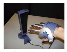
Fig. 1. The P5 glove controller
